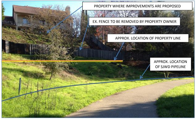
FIGURE 2 – PIPELINE AND PROPERTY LINE RELATIVE LOCATIONS – LOOKING NE
