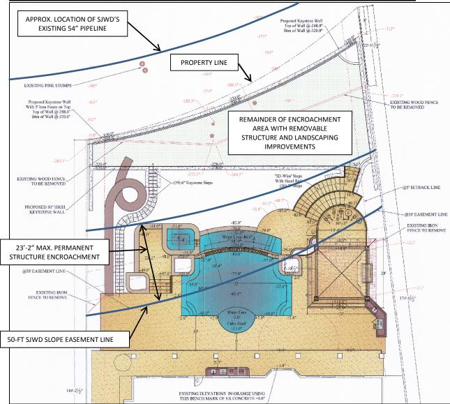
FIGURE 4 – 50-FT SJWD SLOPE EASEMENT – PROFILE VIEW OF PROPOSED IMPROVEMENTS IMPACT
