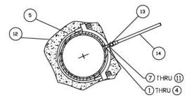
CEMENT MORTAR COATED STEEL MAINS
