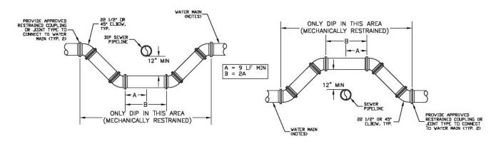
SECTION - WATER MAIN CROSSING UNDER SEWER
