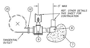
STEEL MAINS TYPE "B" (LATERAL INSTALLATION)
