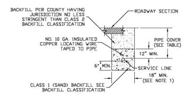
BACKFILL PER COUNTY ROADWAY SECTION HAVING JURISDICTION NO LESS STRINGENT THAN-CLASS 2 BACKFILL CLASSIFICATION 12' NON-METALLIC WATELINE LOCATION TAPE (PROVIDE 2 TAPE PIPE COVER RUNS FOR 16' AND LARGER (SEE TABLE) DIAMETER PIPE) NO. 10 GA. INSULATED 12" MIN. COPPER LOCATING WIRE TAPED TO PIPE -WATER MAIN PIPE DIAMETER + 16" MIN. CLASS 1 BACKFILL SEE BACKFILL CLASSIFICATION
