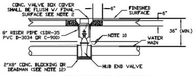
SECTION - HUB END VALVE ASSEMBLY
