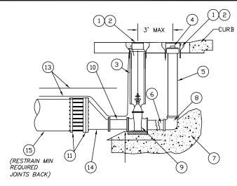
DUCTILE IRON & PVC MAINS TYPE "A" (LONGITUDINAL INSTALLATION)
