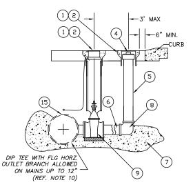
DUCTILE IRON, ASBESTOS CEMENT & PVC MAINS TYPE "B" 12-IN DIA. OR SMALLER (LATERAL INSTALLATION)
