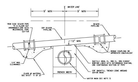
TYPICAL CROSSING DETAIL WATER LINE UNDER SEWER
