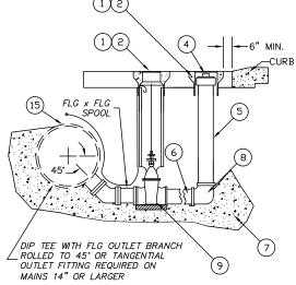
DUCTILE IRON, ASBESTOS CEMENT & PVC MAINS TYPE "B" 14-IN DIA. OR GREATER (LATERAL INSTALLATION)
